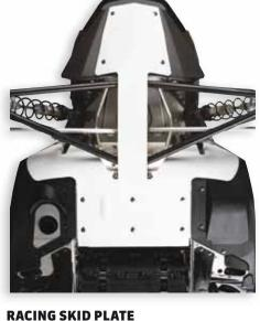
High molecular weight polyethylene embossed with Ski-Doo logo Bulk head wrap industry-first, extended length covers front exchanger, provides maximum lightweight underbelly protection • Relieved A-arms reduce chance of snow buildup.
