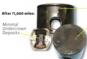
Piston Coating Completely Intact
