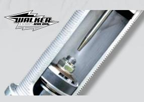
WALKER EVANS COIL-OVER SHOCKS Premium shocks with 16-position compression adjusters and remote reservoirs offer the best in tunability and fade-proof performance. Unique needle design uses hydraulic force at the end of the stroke to eliminate harsh bottoming.
